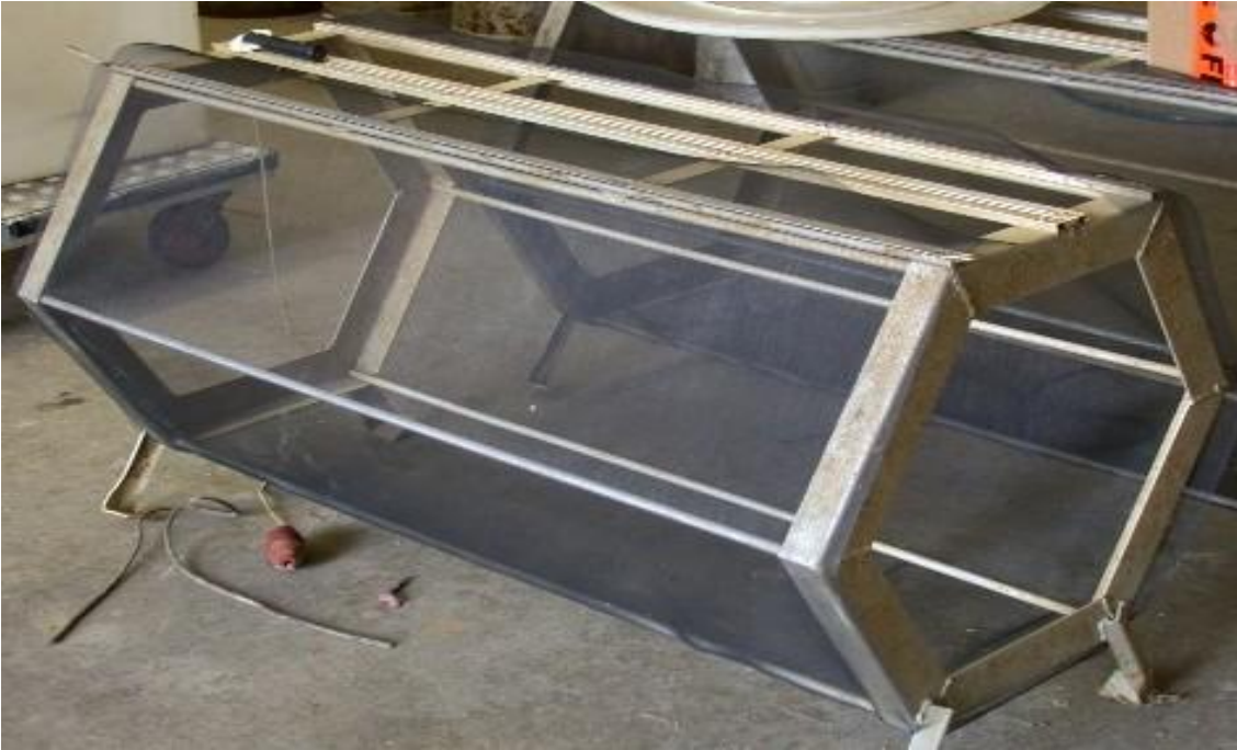
Figure 2.1 Artificial mesh-lined breeding substrate used for the collection of Murray cod eggs from earthen dams at Snobs Creek Fish Hatchery, Eildon, Victoria.
