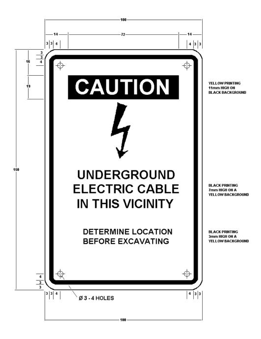
Figure 1. Typical Underground Cable Warning Sign
