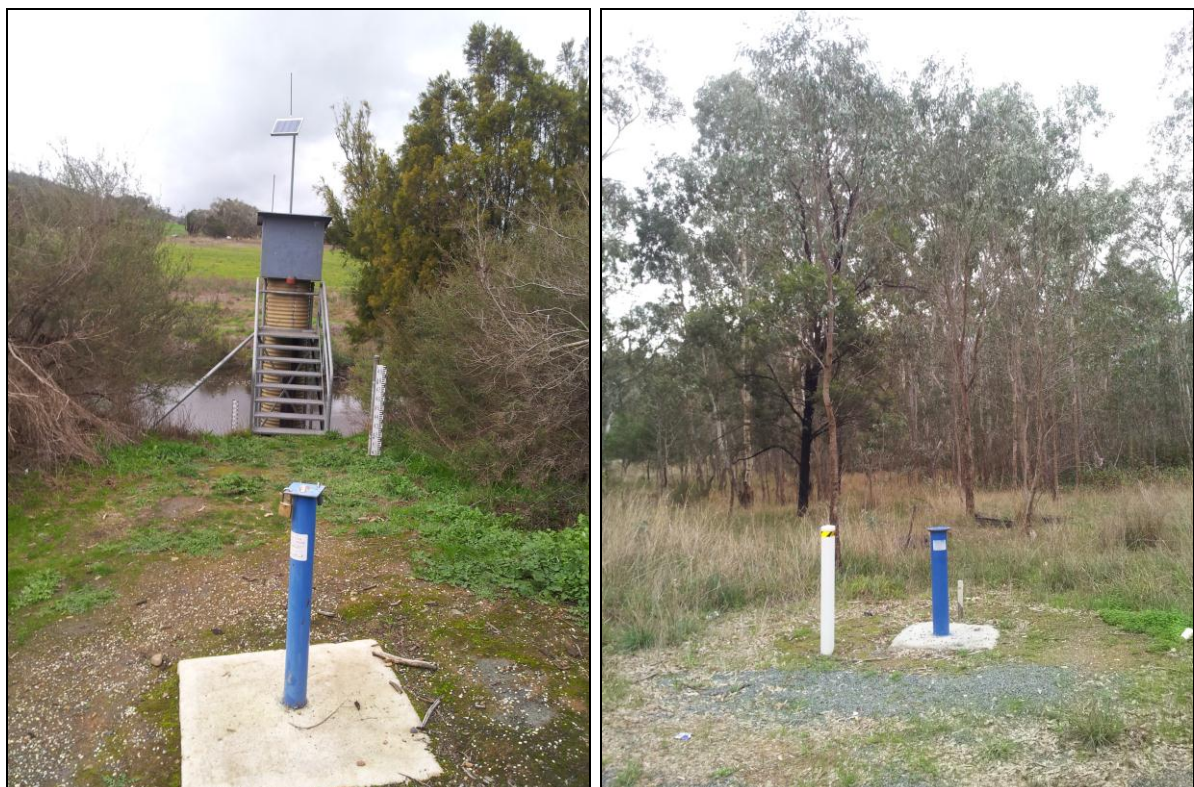
Figure 12 Yea surface water gauge and groundwater monitoring bore at Devlins Bridge and a King Parrot Creek groundwater monitoring bore
