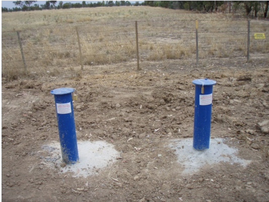
Nested State monitoring bores at Murchison
