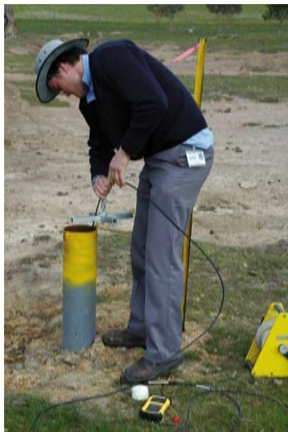
G-MW's Nick McKinley taking a level reading from an observation bore. G-MW's extensive network of observation bores assist in monitoring groundwater levels and assessing the health and rates of recharge of the aquifers in G-MW's region.
