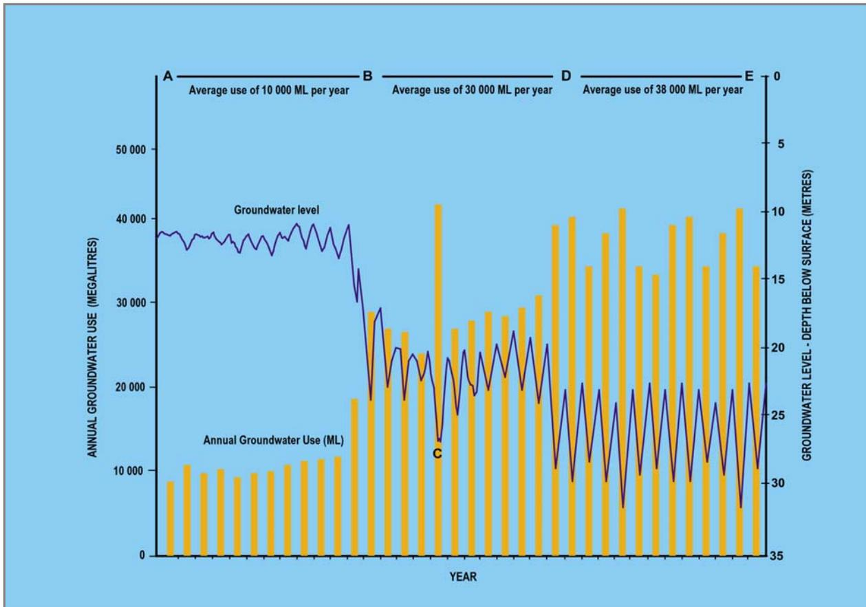
**Figure 3. Typical relationship between use and groundwater levels**
