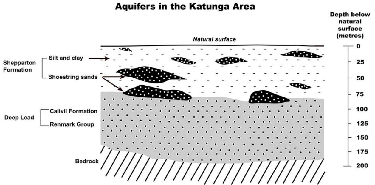
**Figure 1. A cross-section of the aquifers in the Katunga Water Supply Protection Area**
