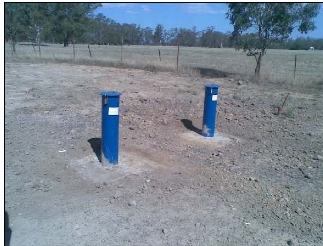
Figure 19 State observation bores
